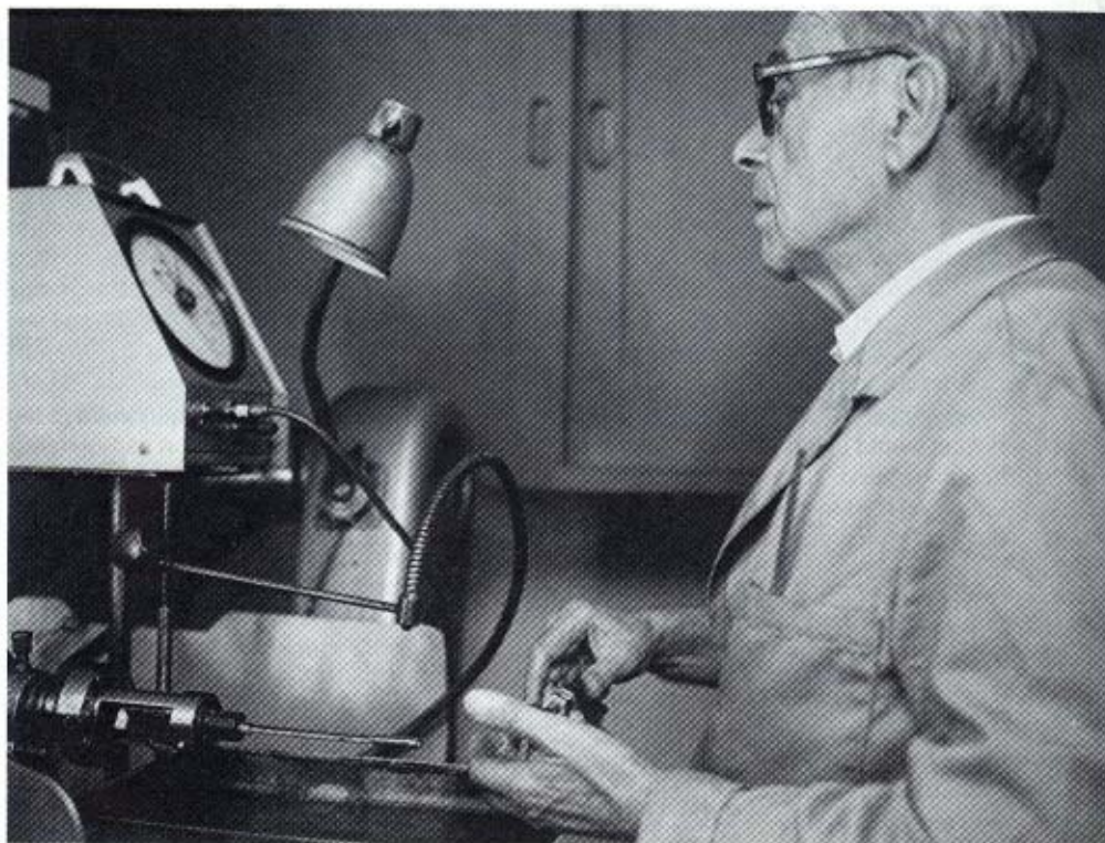
Gauging the bores of a Jacot tool. Note the Mercer Air Gauge.
