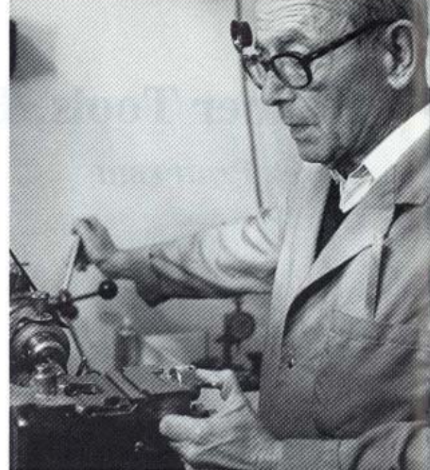
M. Yves Thiébaud, September 1992. Reaming the bores for the runners on a Jacot tool.
