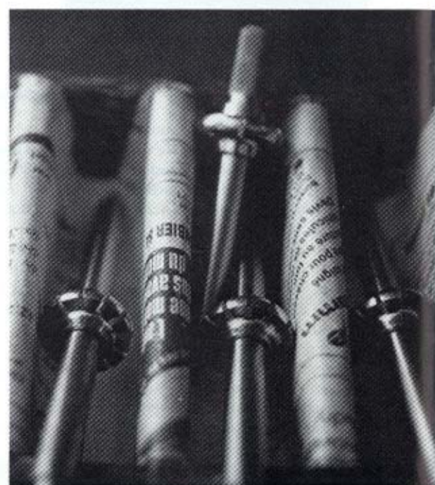
▲ A batch of Jacot tool runners. The notched disc is fitted at an early stage and used to index the notches and flats during manufacture as well as in use for pivot burnishing.
